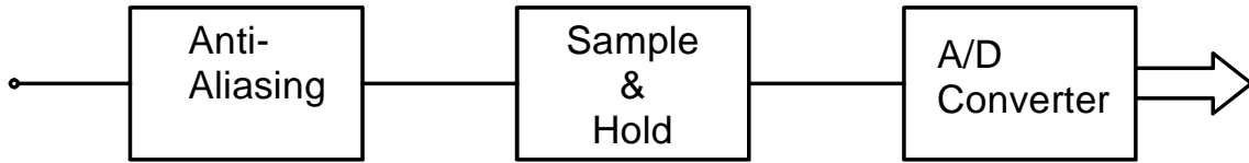
Fig. 1.1.3.13: Usual configuration of a data acquisition channel
